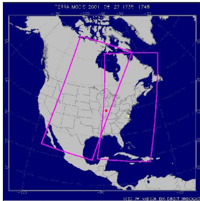
Figure 19. NASA Depiction of Overlapping Swath Width for Consecutive Descending Polar Orbit Passes for the Terra Satellite (NASA-Earth Observatory)
